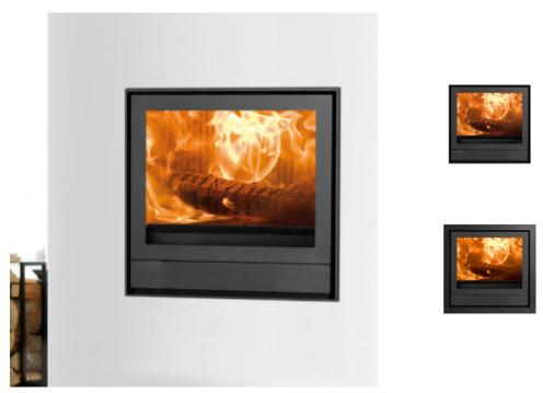
This stove is equipped with white, cast iron, internal, protection plates to reflect heat out into the room; these decrease the heat energy lost up the chimney and to the surrounding masonry, which is especially important for inset stoves. The IQ 43 has a nominal output of 10.5kW, more than capable of heating large rooms that would otherwise be cold. There is also a remote control available to make it that much easier to create a comfortable and cosy environment for all to enjoy.
