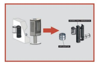
The kit comprises the spigot adaptor for the rear flue exit on the stove, and the snorkel kit which can pass through the wall up to 500mm.
