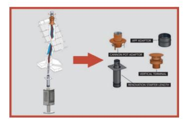
Designed to work with the ACR range of Natural Gas and LPG stoves, this balanced flue kit effectively adapts a conventional flue setup using a flex liner in a masonry chimney, to allow the free space of the chimney to facilitate inbound air required to achieve a balanced flue system.
